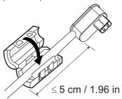
3 Close the ferrite core, snapping the small latches back together.
