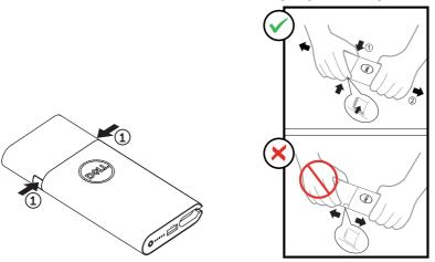
2 While holding onto the latches, pull the power adapter away from the power bank. The power bank and power adapter can now be used separately.
